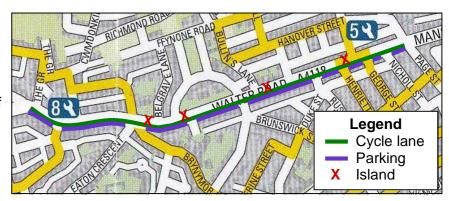
We noted that if parking was provided on the same side as a cycle lane (as shown on the plan above) a buffer between the footway and the cycle lane would be needed to safeguard cyclists from 'dooring'. (A buffer is shown on the Council drawing for the single lane option.)
