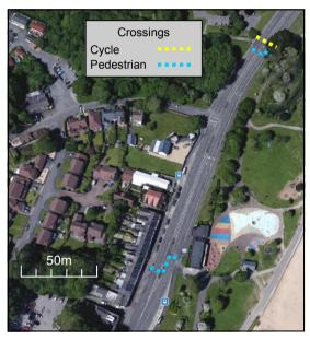
The picture (taken from the paper) shows the crossings. It is about 200m between the two. A car travelling at 30 mph (ie at the speed limit) would take 15 seconds to traverse this distance. This is the key to the proposed phasing.
