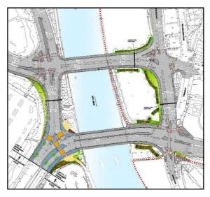
There is sufficient width on the northern bridge for a cycle contra-flow lane and had this been considered at the design stage might have been a possibility. However the junctions at either end present a problem and changes to them would have been necessary. An east-west cycle route on the north bridge was therefore ruled out.
