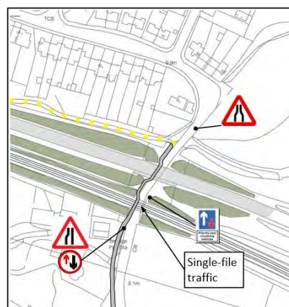
Priority flow system through rail underpass
