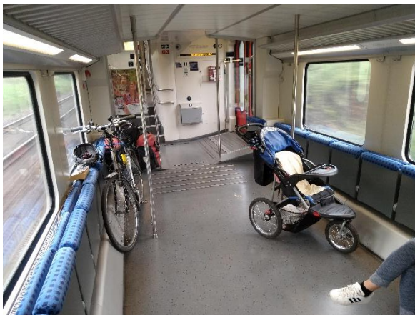
German intercity carriage for bikes, buggies and wheelchairs with tip up seats
