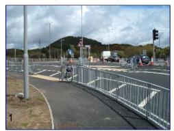
The good part is that for a west bound cyclist, ie travelling towards Swansea, the two sets of lights are clearly visible and appear to default to green in favour of the cyclist, only changing to red when a vehicle approaches the crossing. The bad part is that these lights are not visible to cyclists coming from Swansea, at least not until he or she is on the crossing. The lack of control at the other three crossings is even more dangerous.
