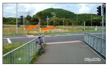
This shows the third crossing, the first with lights. The faces of the yellow control boxes (arrowed) are invisible to an eastbound cyclist. At least one should be turned so that a cyclist can see when it is safe to cross.
